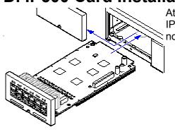
At this stage fit all the internal IP500 cards before powering up the IP500 Office control unit. These processes should be performed with no power to the control unit and following full anti-static precautions.
