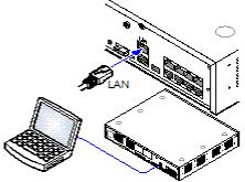
At this stage we will directly connect the Manager PC to the new IP Office control unit. For this the PC will need to be set to a fixed IP address in the same subnet range as the IP Office control unit's default address (192.168.42.1/255.255.255.255).
