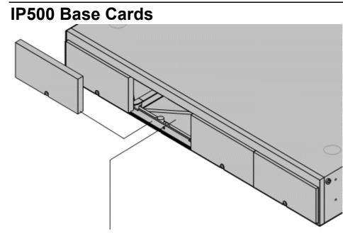
The IP500 control unit has 4 slots for the insertion of base cards. Each base cards includes an integral front panel with ports for cable connections.
