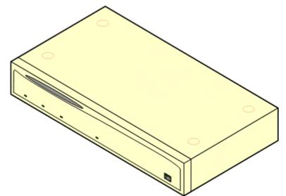
The WAN3 exists in two variants. The original WAN3 only supported a 10Mbps LAN connection and is not supported on IP Office 3.2 and higher. The WAN3 has been superseded by the WAN3 10/100 which supports a 10Mbps/100Mbps LAN connection.
