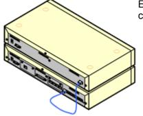
External expansion modules, except the WAN3, connect to the IP Office control unit using a blue 1 meter (3'3") expansion interconnect cable.
