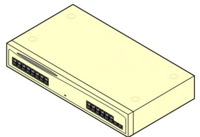
With IP Office 3.1 and higher, the message waiting indication (MWI) on each POT port can be configured for *None*, *On*, *51V Stepped*, *81V*, *Line Reversal A* or *Line Reversal B*. *On* uses the default determined by the system locale. POT ports on a Phone V2 module can additionally be configured for *101V* operation.
