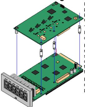
IP500 daughter trunk cards can be fitted to IP500 base cards to provide support for trunk. The daughter card uses the physical ports provided on the front panel of the base card for cable connection.
