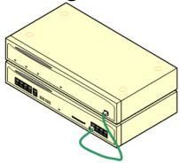
WAN3 expansion modules connect to the IP Office control unit using a LAN cable. It is preferred that the cable is connected directly to the IP Office control unit rather than via any other equipment. A green 1 meter (3'3") LAN interconnect cable is supplied with the module for this purpose though a replacement cross-over cable is required if connecting to an IP412 control unit.
