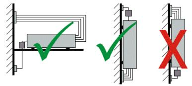
• The Z-shaped bracket **must not be used** as the sole mounting fixture.
