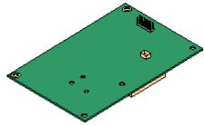
This card can be added to an IP500 base card except the IP500 Legacy Card Carrier base card. The card is a universal card that can be configured in software for E1 PRI, T1 robbed bit, T1 PRI or E1R2. The card is available in single and dual port variants.
