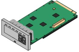
This card provides voice compression channels for use with VoIP calls. The module is available in variants supporting up to 32 or 64 channels. Each card provides 4 initial channels with additional channels being enabled by licenses in the IP Office configuration. The card can be fitted with an IP500 daughter card which then uses the 4 RJ45 ports for connections.
