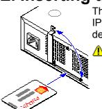
The IP500 uses a smart card feature key dongle. In addition to feature licensing the IP500 control unit uses this feature key dongle to determine various systems defaults such as A-Law or Mu-Law operation, default short codes and trunk settings.
