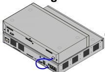
External expansion modules connect to the IP Office control unit using a blue 1 meter (3'3") expansion interconnect cable supplied with the modules.
