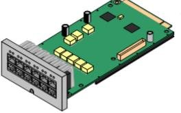
This card has 12 RJ45 ports. The first 8 ports are DS ports for the connection of Avaya digital phones other than IP phones. The card can be fitted with an IP500 daughter card which then uses the additional 4 RJ45 ports for connections.
