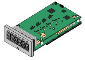
Objective - To fit a IP500 trunk card to an IP500 base
