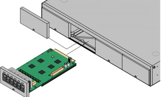
3. Allowing the card to rest against the bottom of the slot, begin sliding it into the control unit. When half inserted, check that the card rails have engaged with the slot edges by trying to gently rotate it. I the card does rotate remove it and begin inserting it again.
