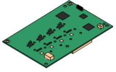
This card can be added to an IP500 base card except the IP500 Legacy Card Carrier base card. It allows that base card to then also support 4 analog loop-start trunks.
