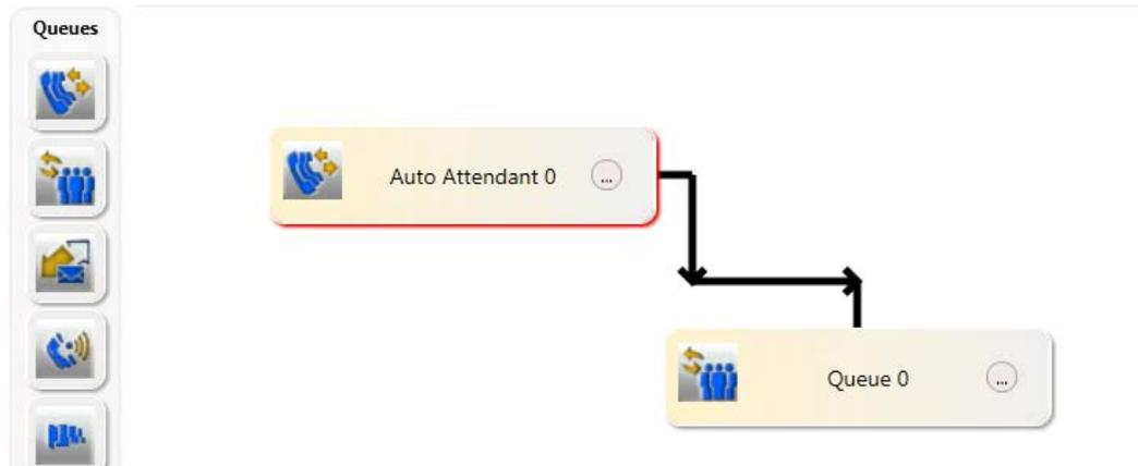
Objects can be moved around the canvas by drag and drop. The currently selected object will have a red-coloured shadow. The line and arrow shows the connection between objects and the direction. The above example shows that 'Auto Attendant 0' can overflow a call to 'Queue 0'
