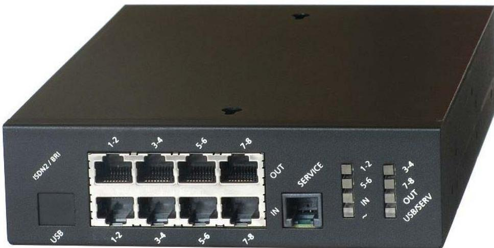
From the ISDN NT unit, the BRI line must first be connected to the IN ports of the recording box. The OUT ports on the recording box will then be connected to the PBX as illustrated with the diagram below. Standard network cables are used for both connections.
