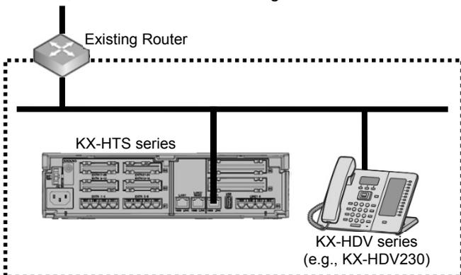
2. KX-HDV series will be registered to KX-HTS series automatically. An extension number is displayed on the LCD of KX-HDV series.
