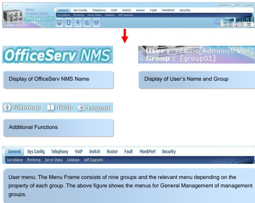
Figure 2.5 configuration of Menu Frame
