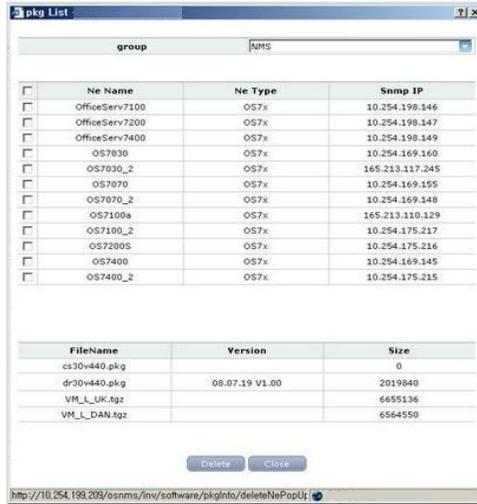
**Figure 5.5 Package Information Management Window for Deleting Files from NEs**
