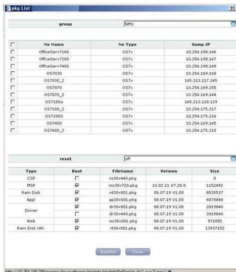
Figure 5.4 Package Information Management Window for Changing the Boot File Option for Multiple Files
