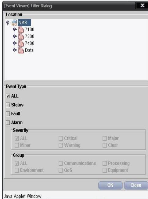
Select NE to be displayed from the 'Location' box, fill check marks in the boxes of Event Type, Severity or Event Group to be received, and click the **[OK]** button.
