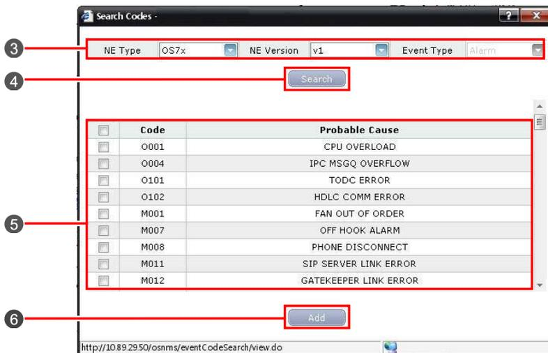
Figure 6.8 Audible Alarm Codes Window
