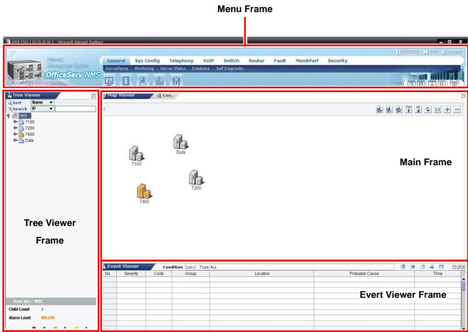
Figure 2.4 Configuration of OfficeServ NMS Frames
