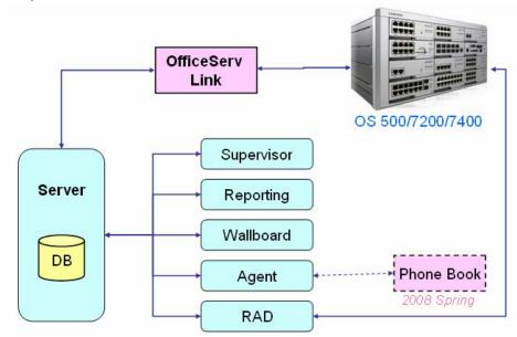
Avaya's Compact Contact Center (CCC) provides the user with the necessary tools to facilitate the management of call traffic. The diagram below shows the concept:
