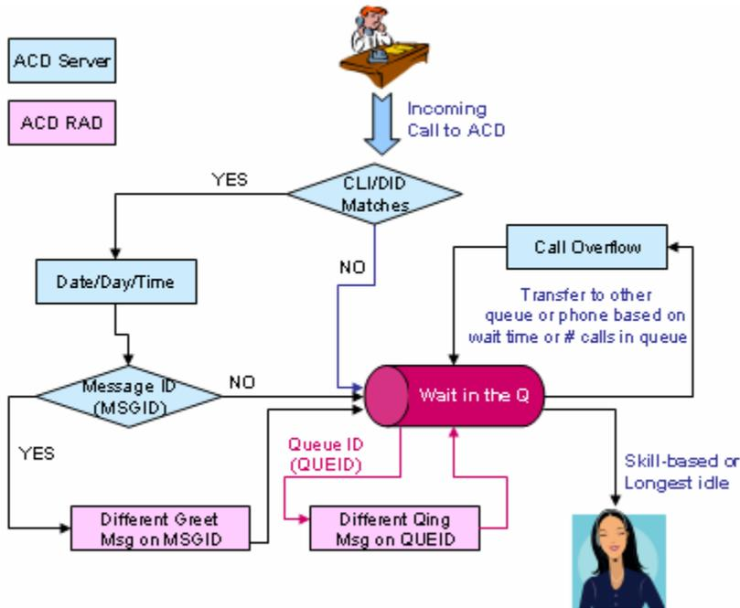
The following figure illustrates the call flow between ACD Server, IVR and Agent. When a new call arrives at ACD gateway port, if IVR routing is configured, the call is routed the IVR. In the IVR, the target split is determined based on the caller's input via DTMF digits. Integrated with customer DB, the caller's personal information such as customer ID, customer level, and customer type is searched, authorized and transferred to the Agent program.
