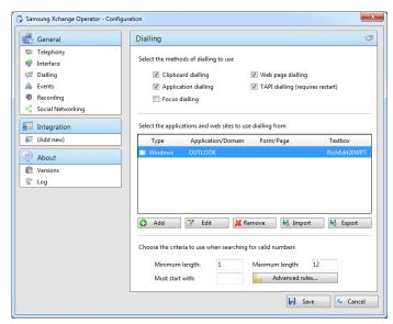
to applications that you have told it about), TAPI dialing (where any application that supports Microsoft TAPI can dial through Samsung Operator ) and Focus dialing (dynamically recognize any numbers in textboxs that looks like the phone numbers and allows to dial that number out).
