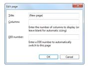
To specify a particular number of columns for displaying the extensions, enter the number into the "Columns" text box or leave it blank to let Operator resize and arrange them automatically.
