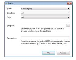
The Program box allows you to select which executable to run. This box should be left blank to load an internet browser.
