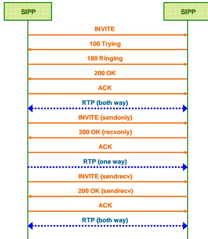
Figure 6. Hold/Resume between SIP Terminals
