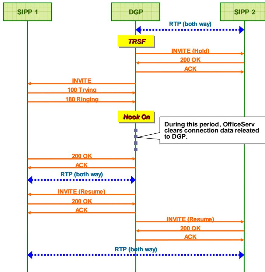
Figure 8. Blind Transfer by DGP as a Transferor
