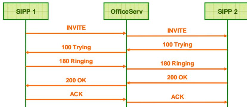
Figure 4. Basic Call Setup Flow between SIP Stations
