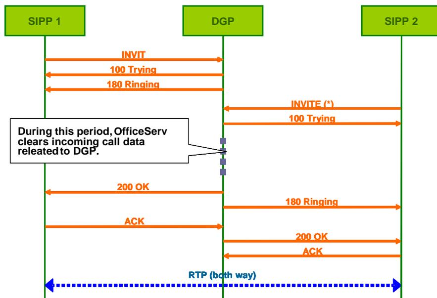
Figure 10. Call Pickup from DGP by SIP Station
