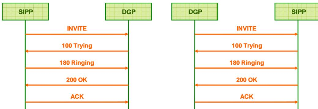
Figure 5. Basic Call Setup between SIP Station and DGP
