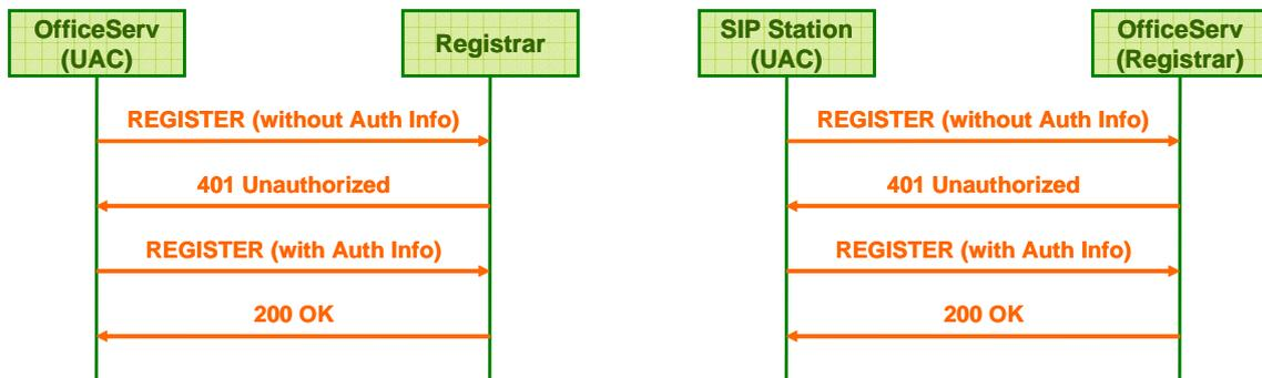
Figure 3. Trunk Mode Registration vs. Station Mode Registration
