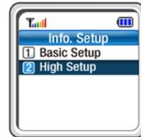
If **High Setup** is selected, the following input procedure is added. (In this mode, wireless LAN security must be disabled for upgrade)
