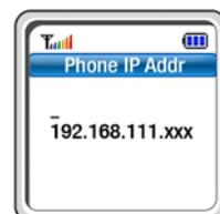
After entering the IP address that corresponds to the same subnet as the OfficeServ system connected to SMT-R2000 and has no conflict with the subnet, press the **[OK]** button to complete the input procedure of High Setup. After that, select Basic Setup and continue the following steps.
