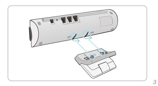
When installing SMT-R2000 to a wall, fix two screws on the wall using a plastic anchor and fit the two holes on the rear side of the support with the screws, and then move the SMT-R2000 downward to fix:
